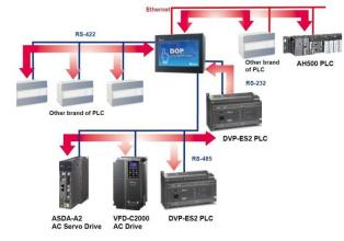
Remote connection for monitoring, visualization and control of the system. This by means of a computer or from your cell phone. Since it has the technology to connect to VNC, you can also configure the ports to perform MODBUS RTU and MODBUS TCP/IP. communications.
