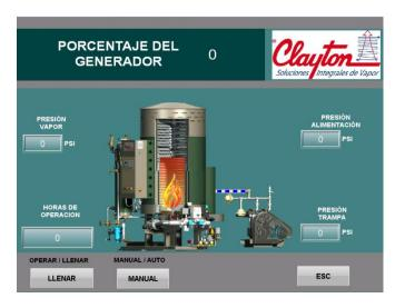
2.- Integration to the communication system through Ethernet through a VNC, to have access to the monitoring of the Clayton Steam Generators.
