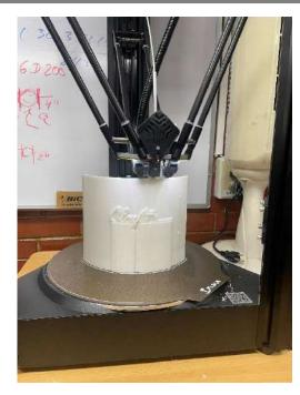
The next step is to put the 3D printer or printers to print the model, for the development of this prototype it is made up of several parts that have to be printed independently and once all the pieces are ready they stop for a process of detailing and cleaning them
